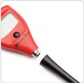
The HI1271 pH electrode can be easily replaced. Just unscrew the electrode from the meter body and screw on a new one.
